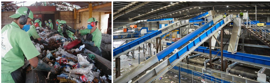
Figure 1: Mixed-waste MRF manual screening conveyor (left) and large scale Advanced MRF operated by Cleanaway in Melbourne (right)
