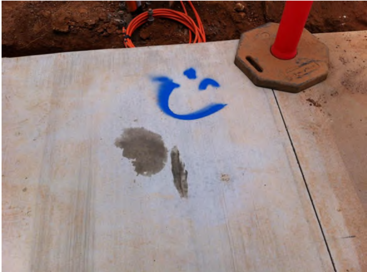
Image 2: Pressure wash did not remove graffiti, cooking oil or motor oil but chewing gum was removed
