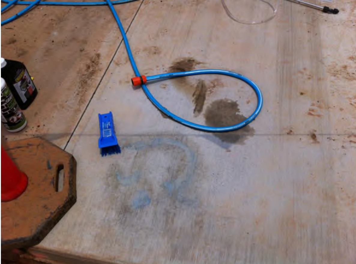
Image 3: Graffiti remover also appeared to remove concrete sealer
